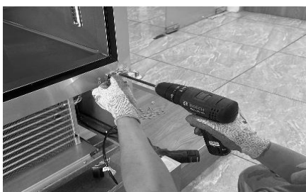
C. Disassemble the bottom right hinge
